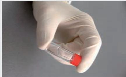
5. Dissolve substrate in cap by gently shaking the cuvette
