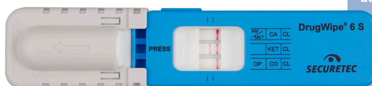
A DrugWipe 6 S with a positive ketamine test result.
