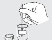
8. Open the buffer container, immerse the spatula in the buffer solution and stir for 5 seconds.
